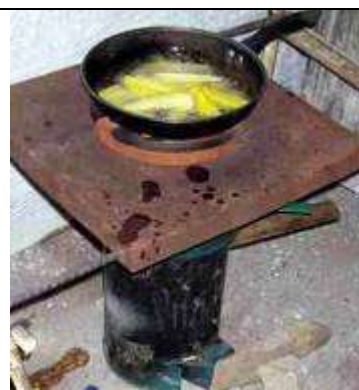
A Champion reactor made in Mozambique with a fixed stand for the pot (Photo: Carmel Lloyd)
